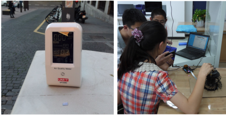
Figure 1. Schoolchildren collecting and scanning PM2.5 particles using a DIY AFM. The image on the left shows a piece of a DVD disk without protective layer placed outdoors (shown next to an air quality meter for reference). In the right, the AFM is being used to image PM2.5 particles.
